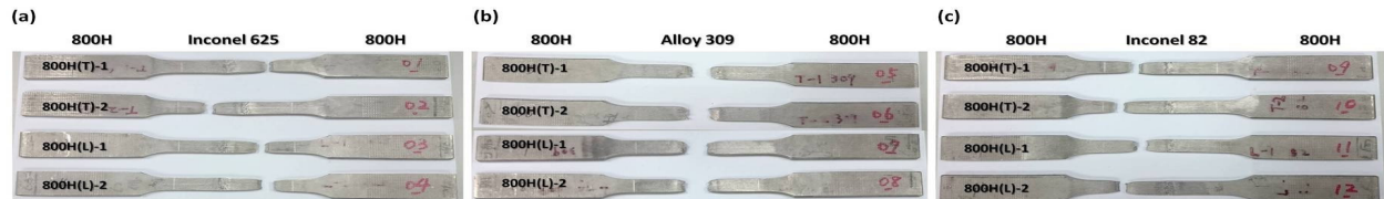
Fig.11. Ruptured specimens after tensile testing : (a) Inconel 625 weld metal, (b) Alloy 309 weld metal and (c) Inconel 82 weld metal.
